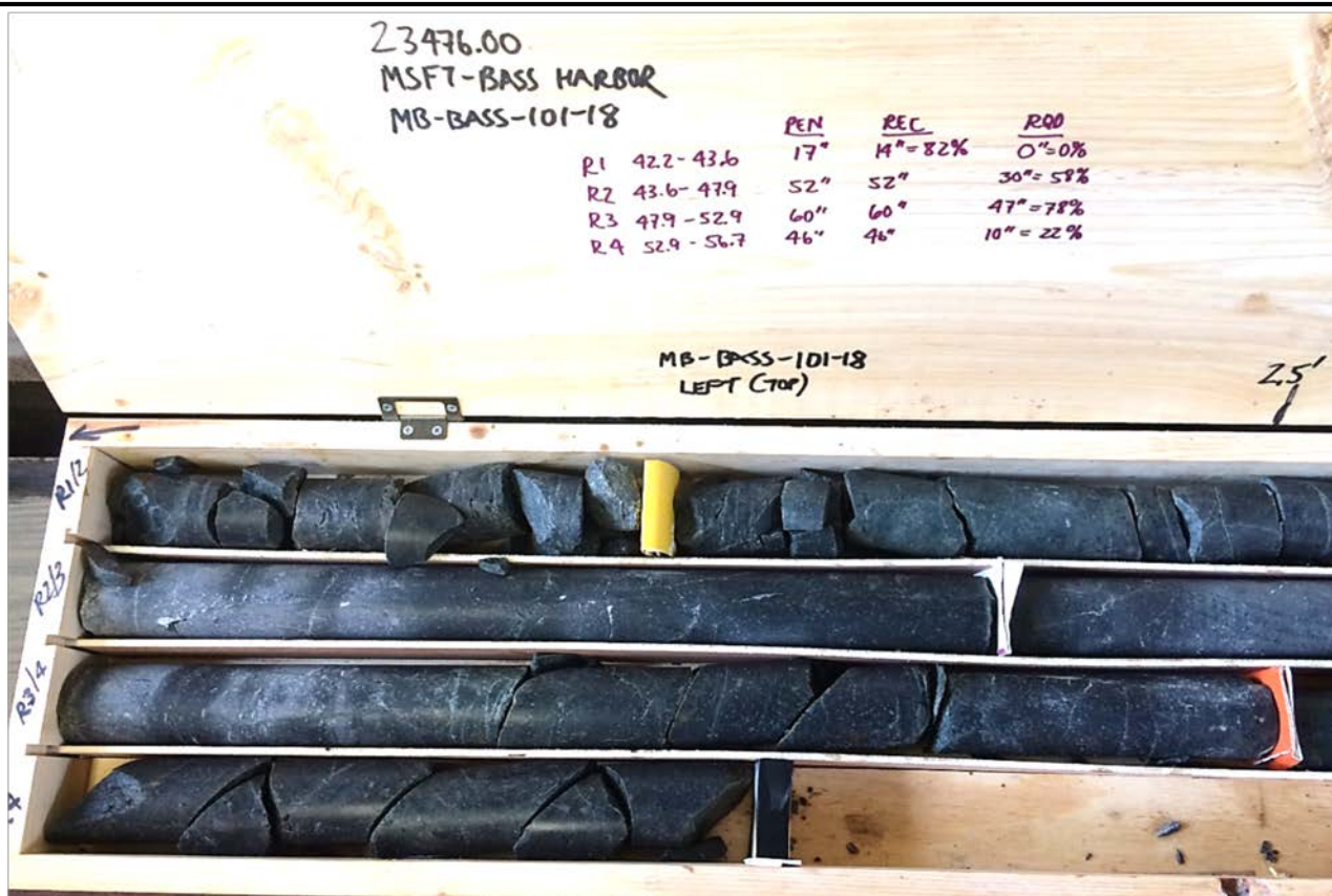
Photo 1: Core box containing wetted rock core from test boring MB-BASS-101; left side of core box (top portion of cores). Slots from top to bottom:
