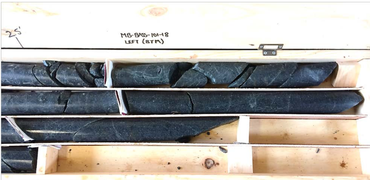
Photo 4: Core box containing wetted rock core from test boring MB-BASS-101; right side of core box (bottom portion of cores). Slots from top to bottom:
