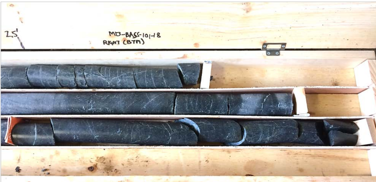
Photo 2: Core box containing wetted rock core from test boring MB-BASS-101; right side of core box (bottom portion of cores). Slots from top to bottom:
